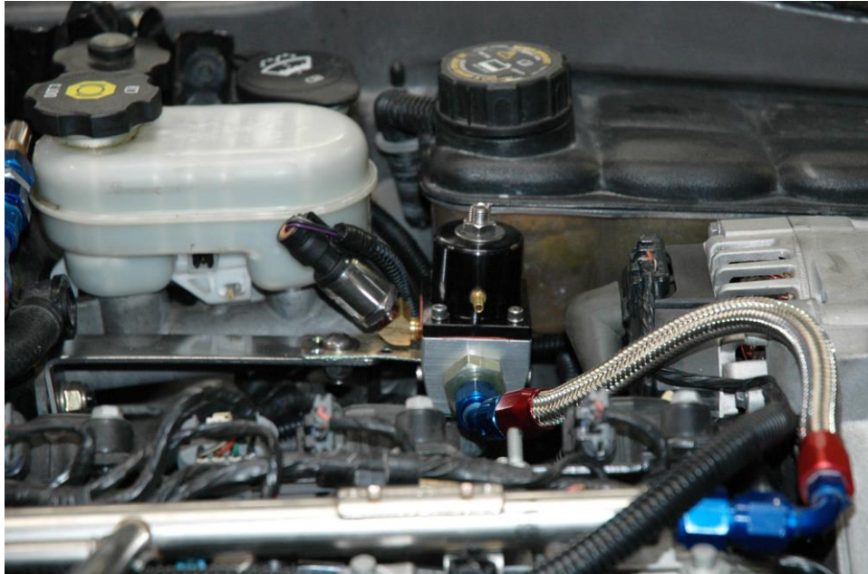
(BRACKET MOUNTED ON BRAKE BOOSTER)
