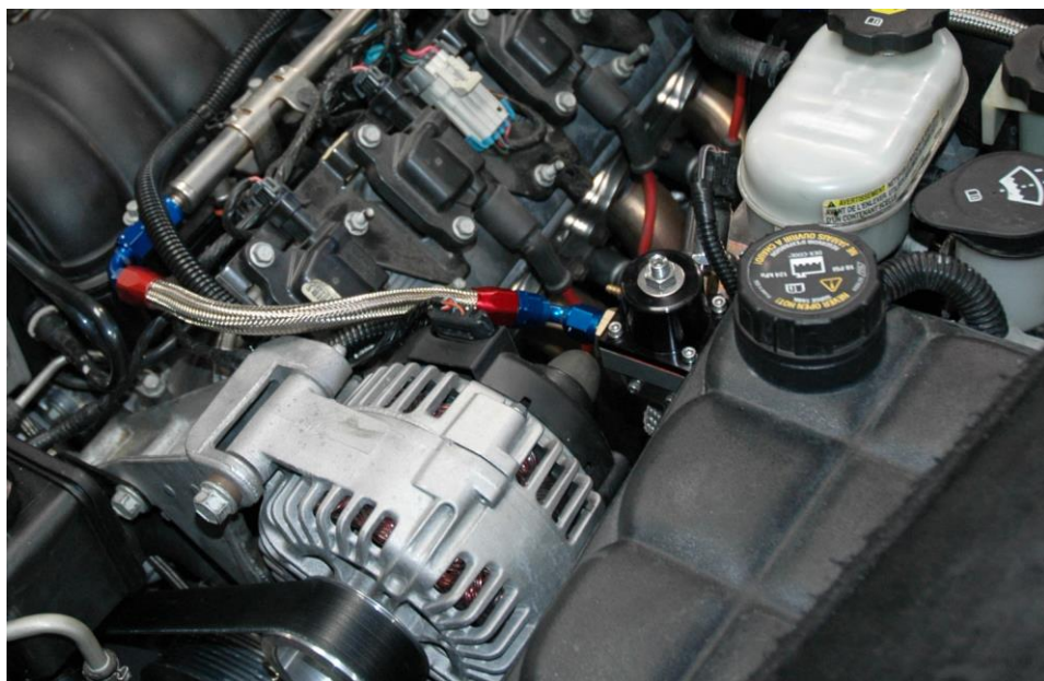
(RETURN LINE ATTACHED TO FUEL RAIL AND REGULATOR)
