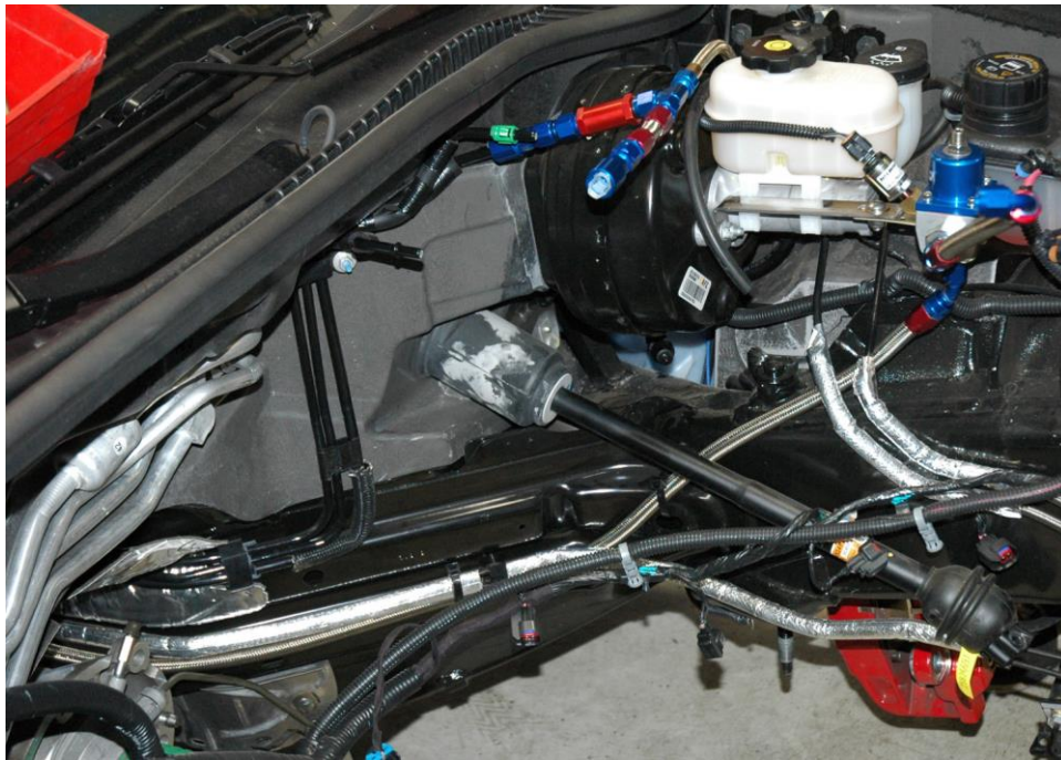
(EXAMPLE OF RETURN LINE SECURED OUT OF THE WAY)
