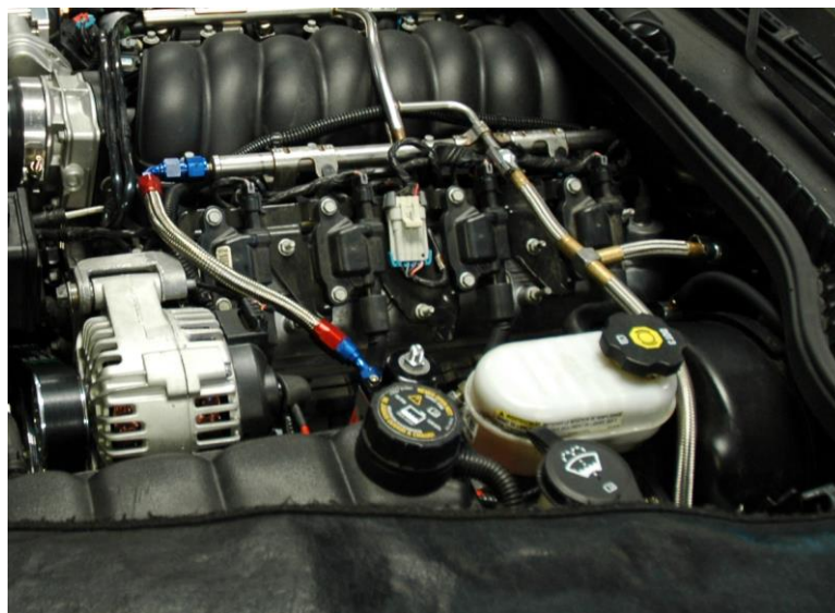
TFE BRAIDED FEED "T" FUEL LINE IN PLACE
