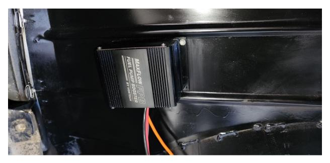
4 Grind a small section of the panel to attach the ground wire with the 3/8" self-tapping screw.
