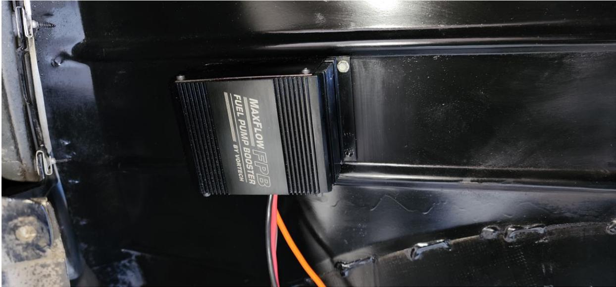
4 Grind a small section of the panel to attach the ground wire with the 3/8" self-tapping screw.
