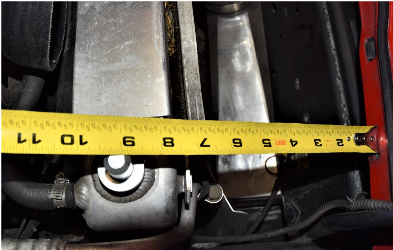
PROPER RADIATOR LOCATION FOR AIR BRIDGE AND TOP SHROUD INSTALLATION
