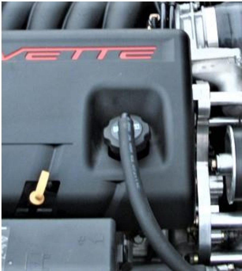
SUPPLIED OIL CAP and VENT HOSE INSTALLED ON STANDARD C6
