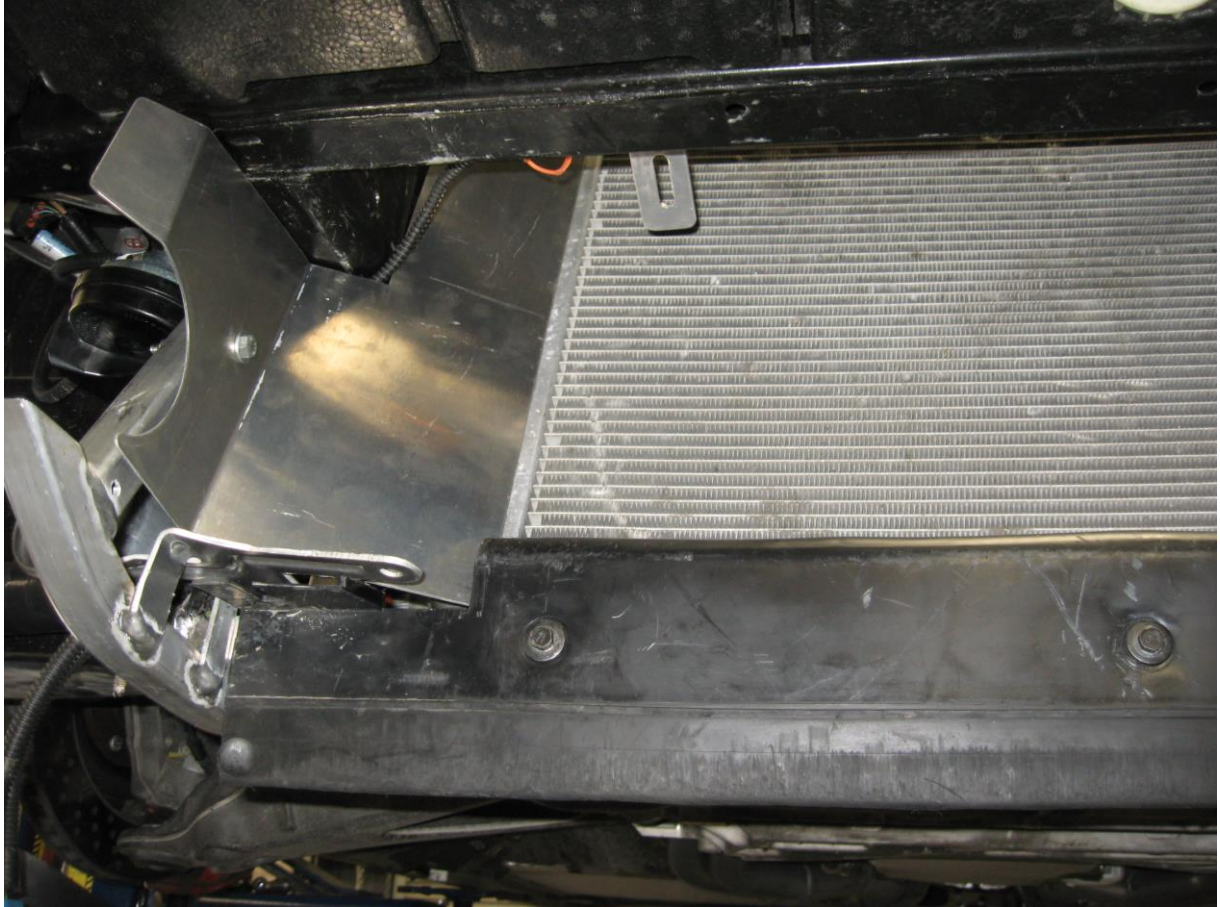
(PASSENGER SIDE PANEL INSTALLED)
