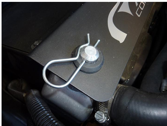
(LEFT AND RIGHT COTTER PINS INSTALLED)
