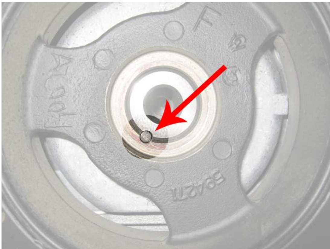
(PIN INSTALLED IN CRANKSHAFT AND BALANCER)
