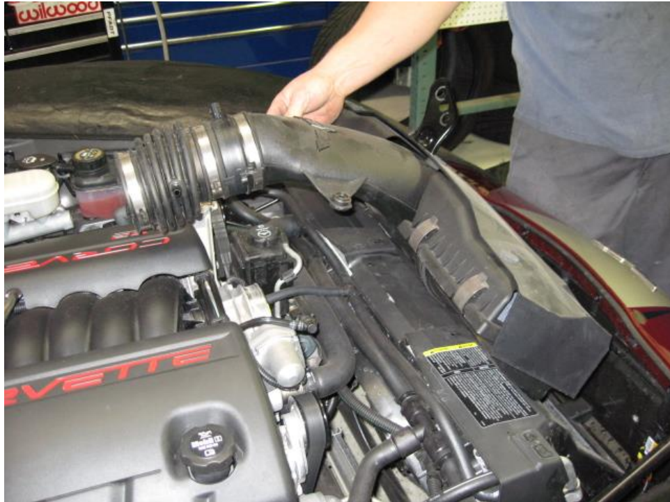
VALVE COVER BREATHER HOSE, MAF CONNECTOR AND AIR FILTER ASSY REMOVED
