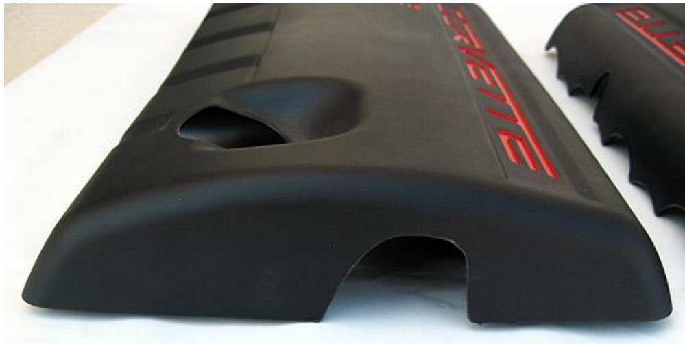
(PASSENGER SIDE COIL COVER TRIMMED)
