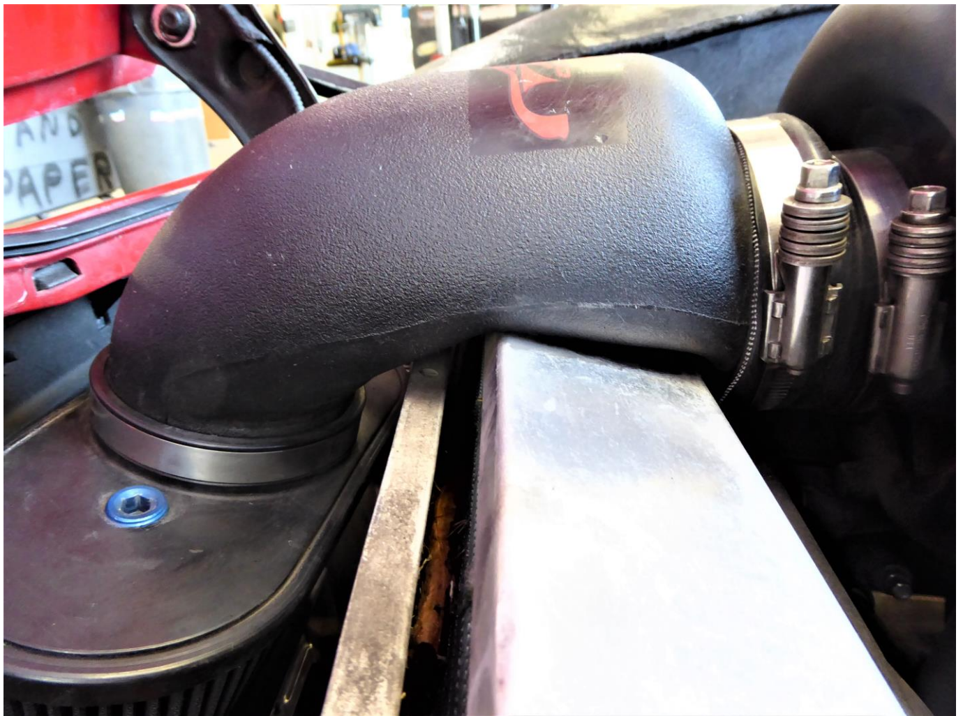
AIR BRIDGE INSTALLED OVER RADIATOR (aftermarket oversized radiator shown- stock radiator
