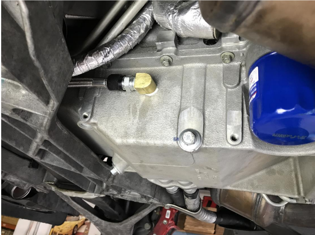
(OIL DRAIN FITTING INSTALLED IN DRY SUMP OIL PAN)
