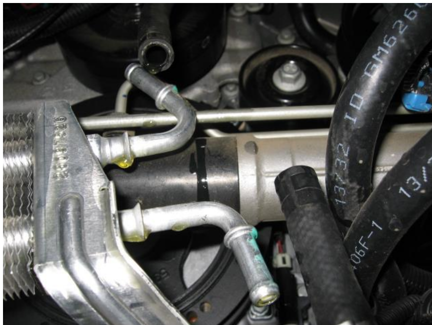
(POWER STEERING COOLER AND HOSES)
