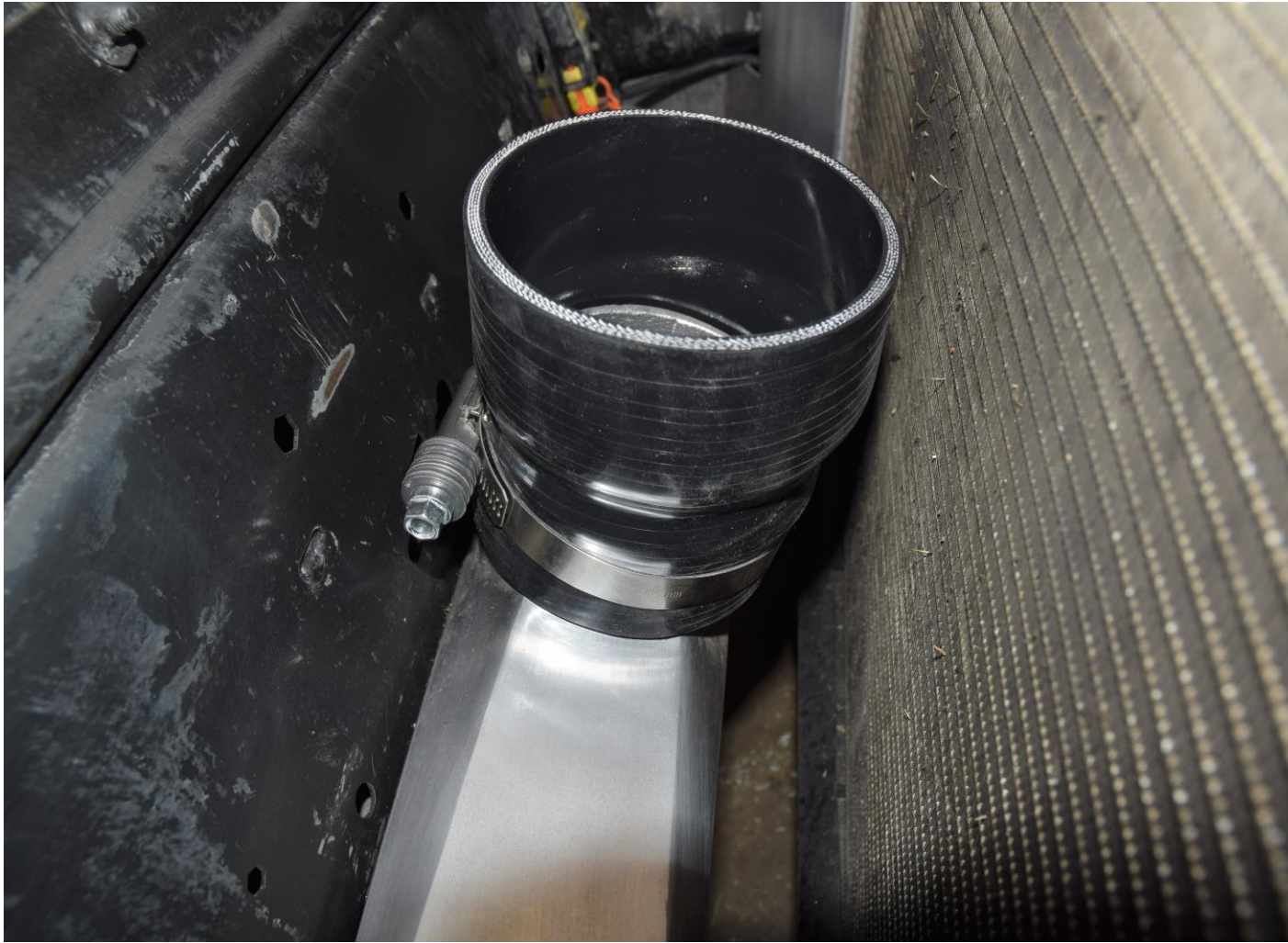
ANGLED COUPLER BETWEEN INTERCOOLER AND MAF TUBE
