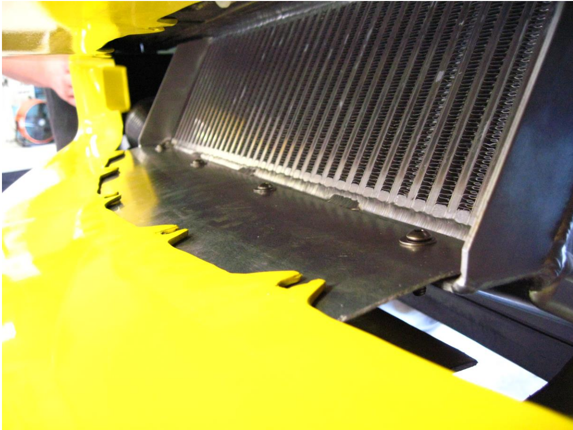
INTERCOOLER DUCKBILL SHOWN INTERFACING WITH FRONT FASCIA
