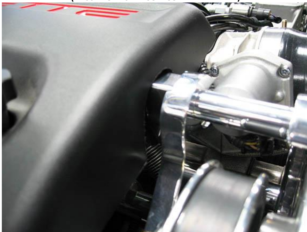
(TRIMMED PASSENGER SIDE COIL COVER INSTALLED)
