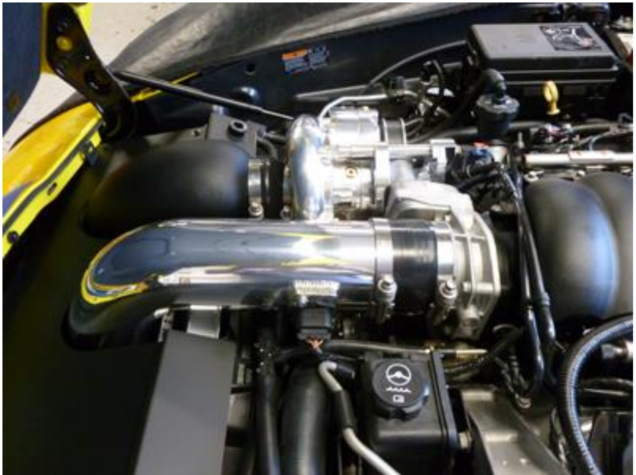
(INLET TRACT ASSEMBLED LS7 AND LS3)
