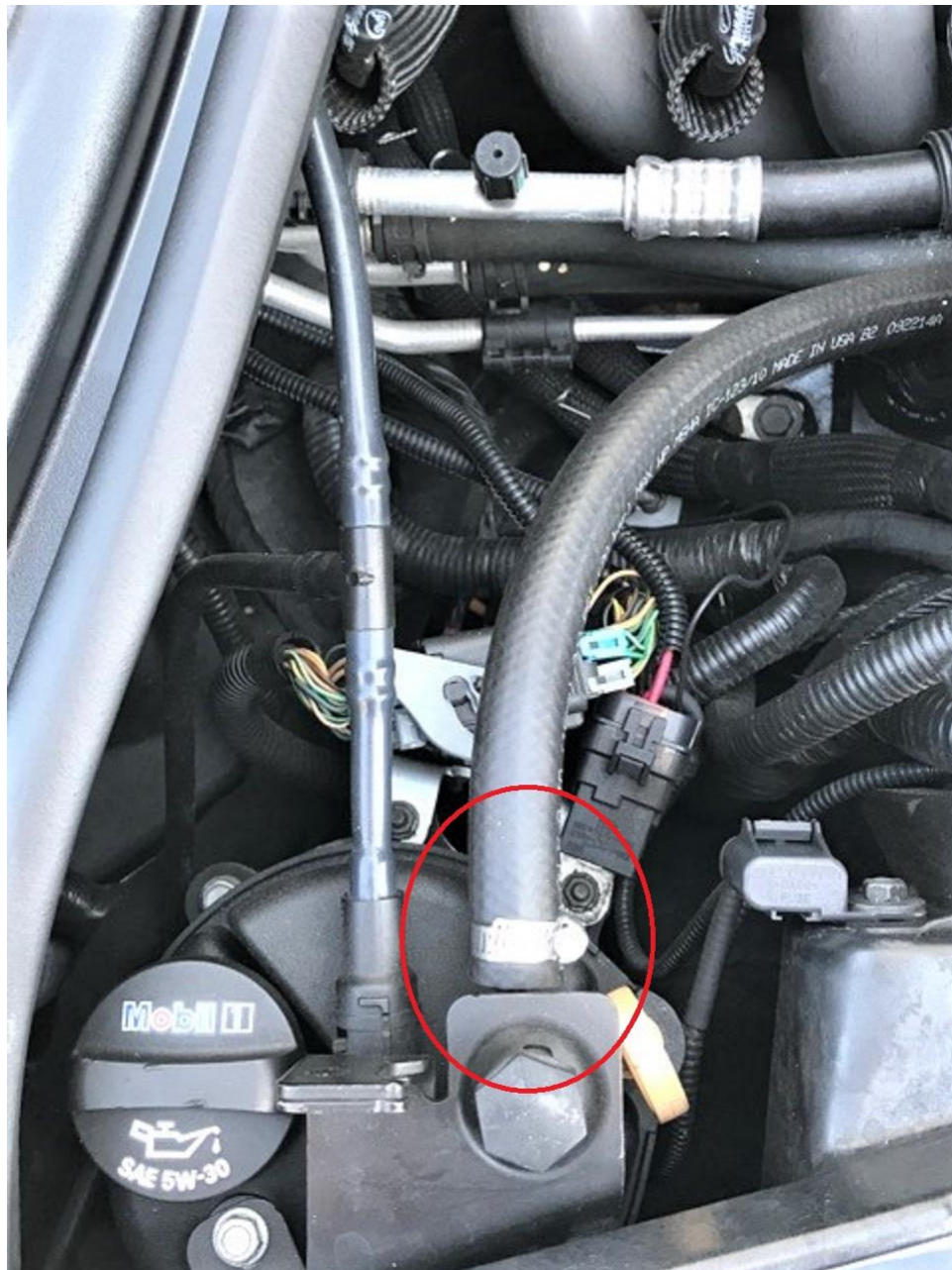
VENT HOSE ON Z06 DRY SUMP
