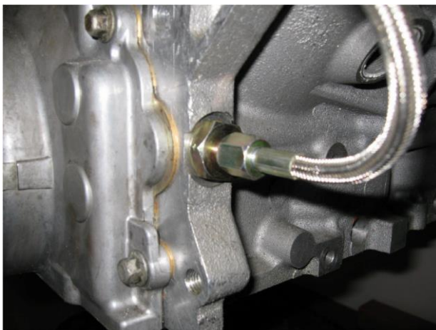
(OIL FEED LINE AND FITTING LOCATION AND OIL LINE ROUTING)
