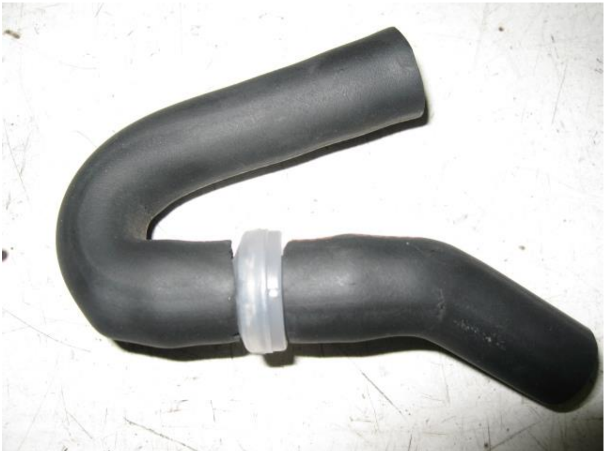
(CHECK VALVE INSTALLED IN VENT TUBE FROM VALLEY COVER)
