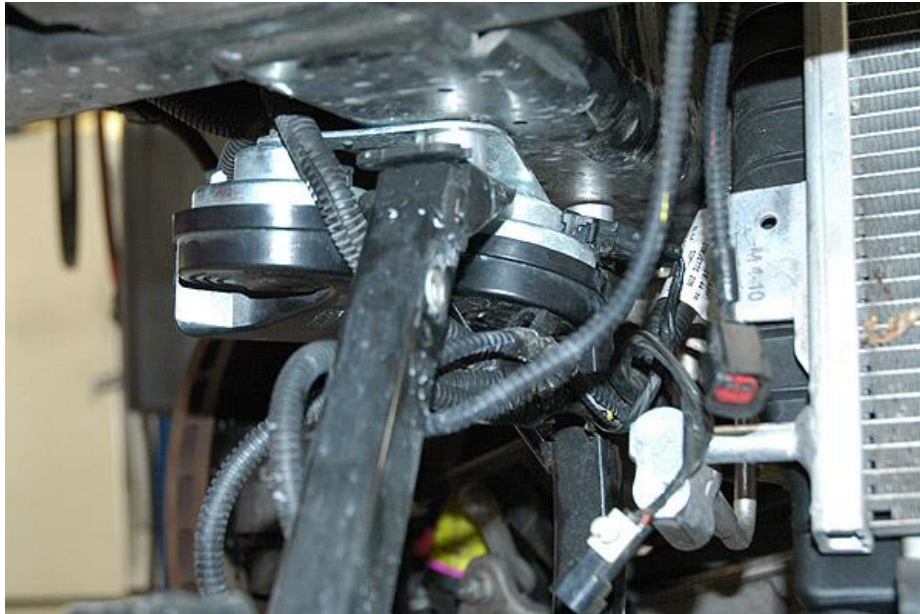
(HORN ASSEMBLY INSTALLED ON PASSENGER SIDE)
