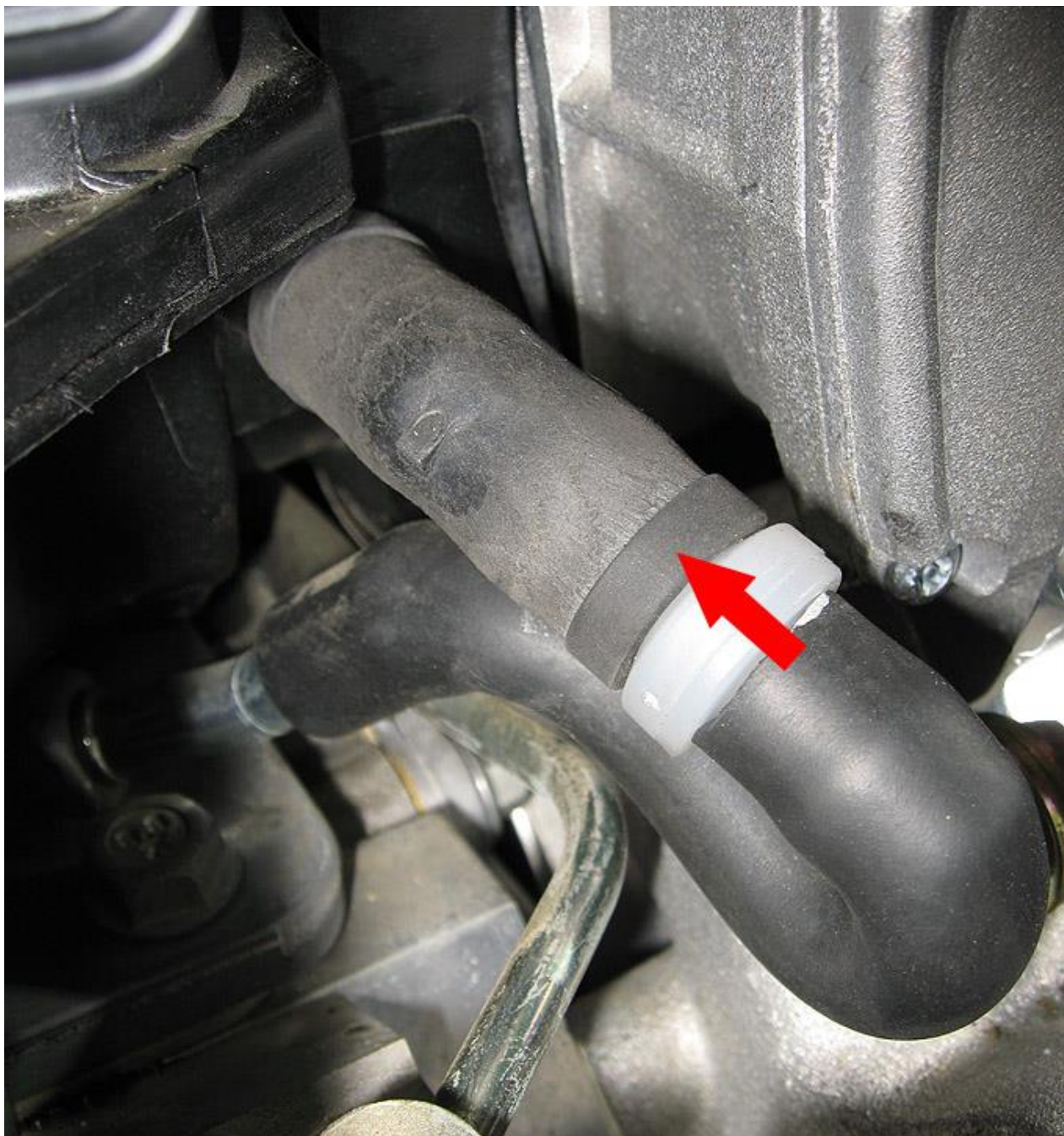
(VENT TUBE WITH CHECK VALVE INSTALLED, AIRFLOW DIRECTION INDICATED)
