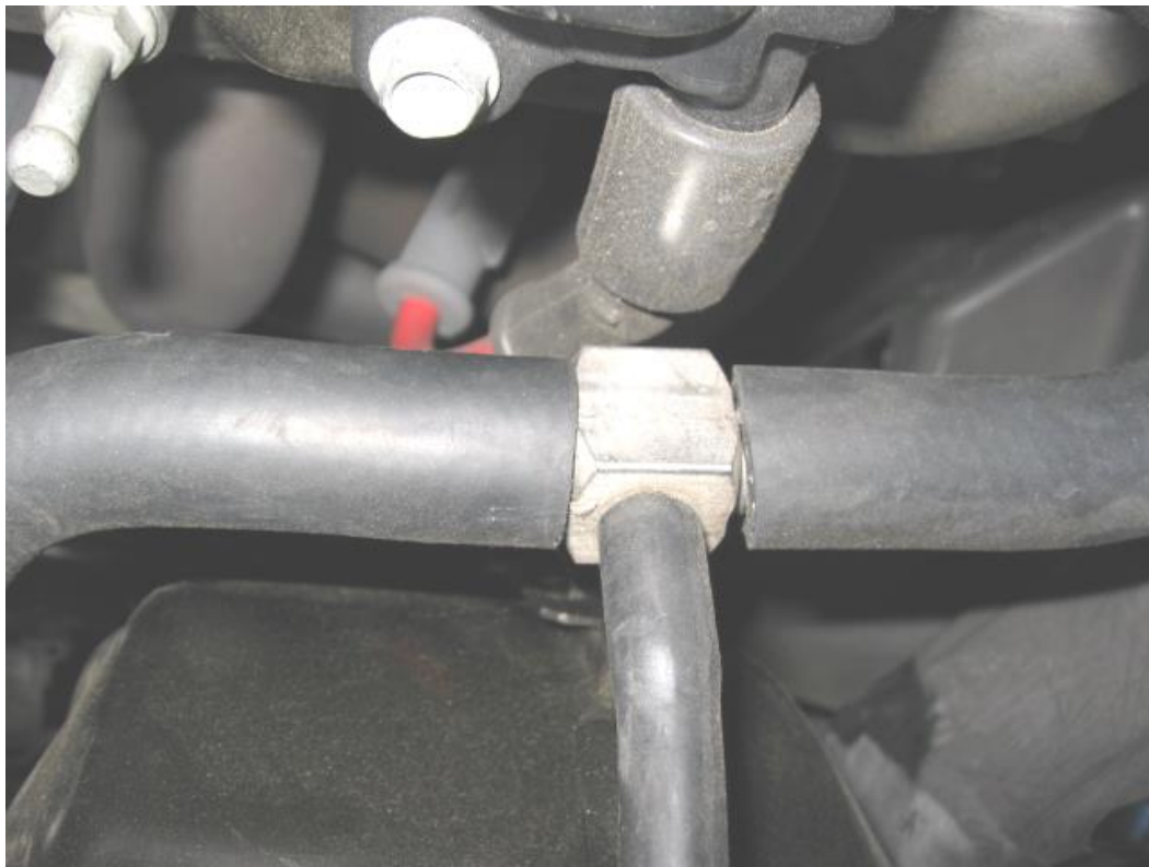
(STAINLESS "T" INSTALLED IN BRAKE BOOSTER HOSE)
