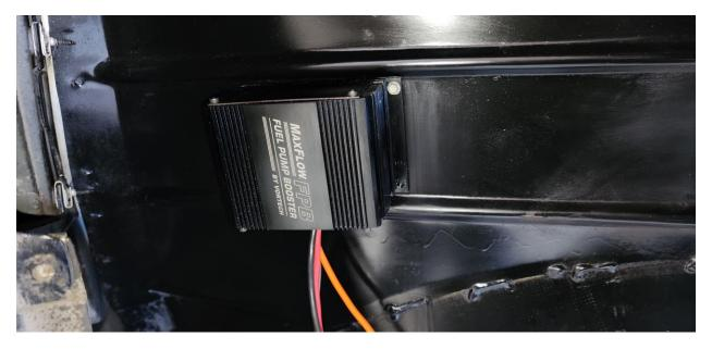
3 Grind a small section of the panel to attach the ground wire with the 3/8" self-tapping screw.
