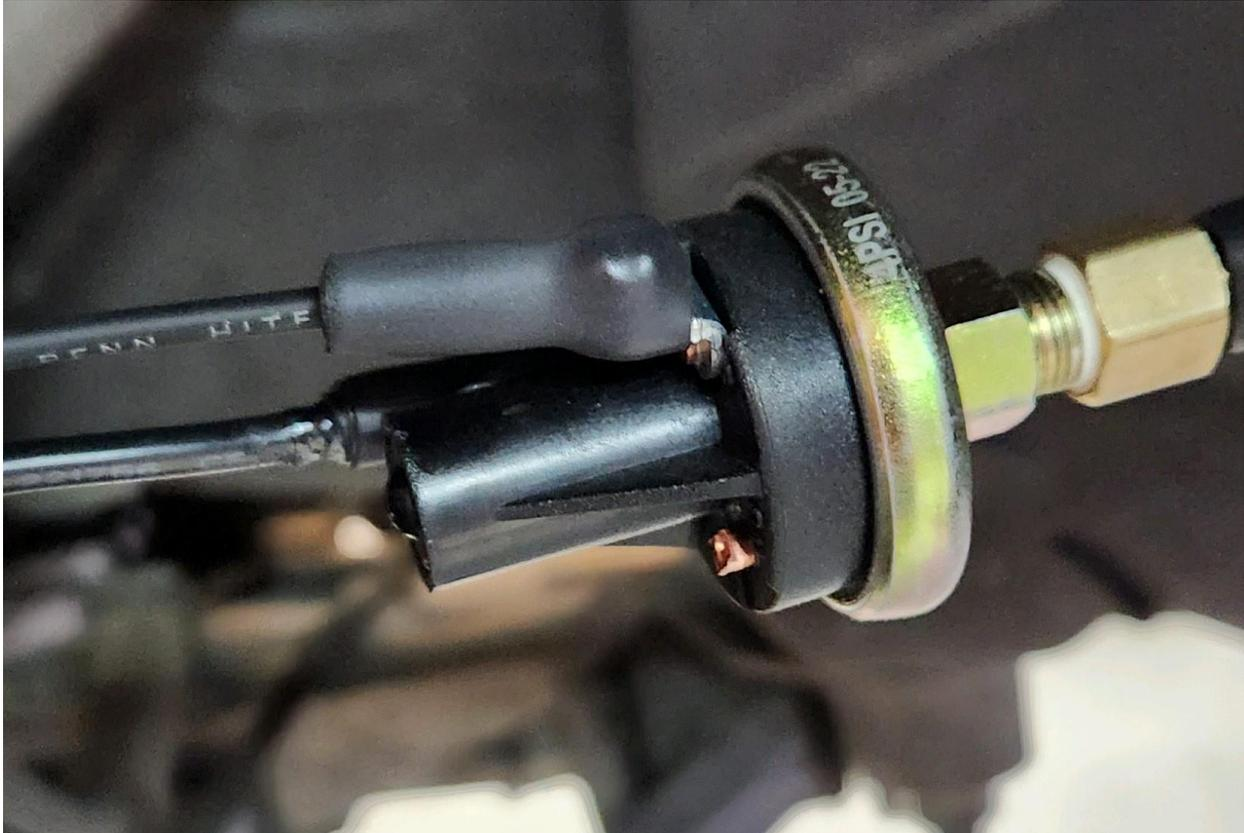
8 Attach the supplied piece of vacuum hose to the barb fitting on the pressure switch. This hose will “T” into the power brake hose along with the blowoff valve hose. The switch can be located anywhere around the fender opening, near the brake booster.
