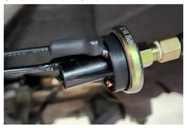
8 Attach the supplied piece of vacuum hose to the barb fitting on the pressure switch. This hose will "T" into the power brake hose along with the blowoff valve hose. The switch can be located anywhere around the fender opening, near the brake booster.
