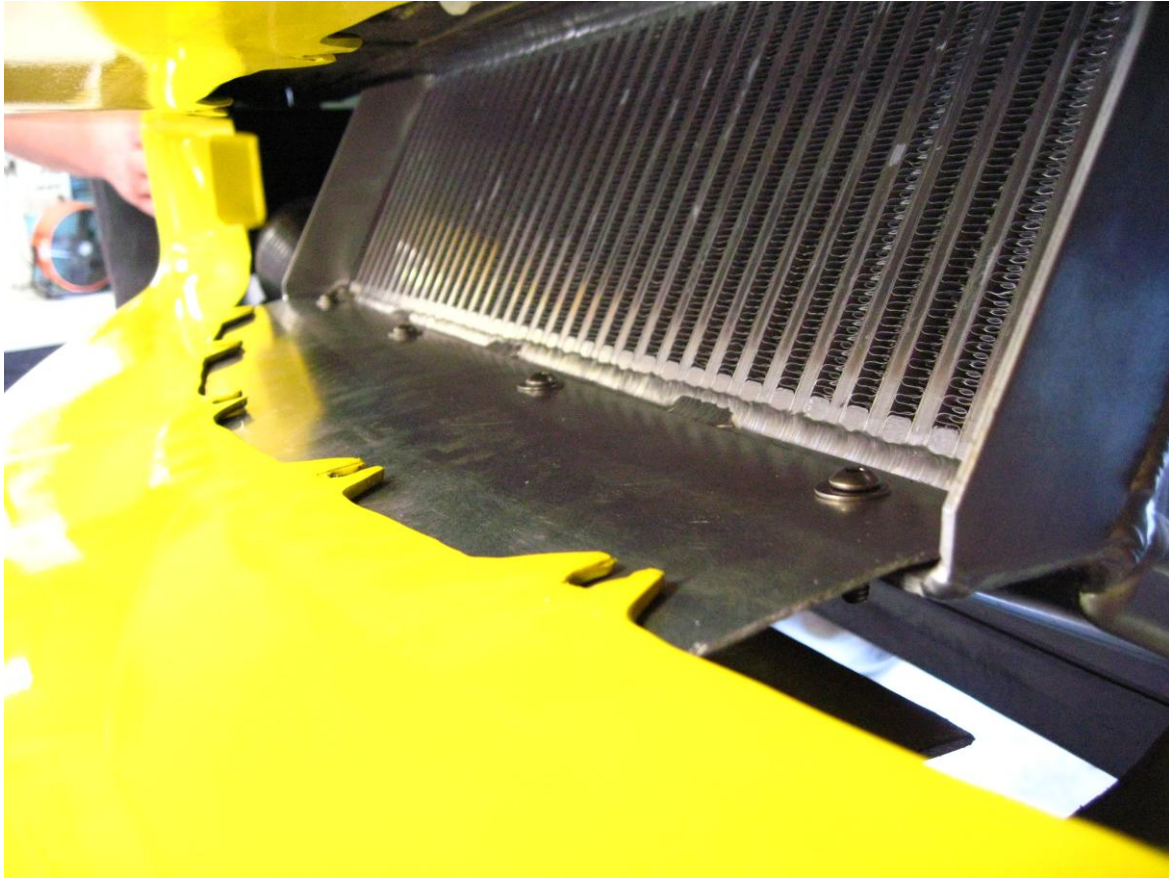
INTERCOOLER DUCKBILL SHOWN INTERFACING WITH FRONT FASCIA (GRILL IS NOT INSTALLED FOR CLARITY ONLY)
