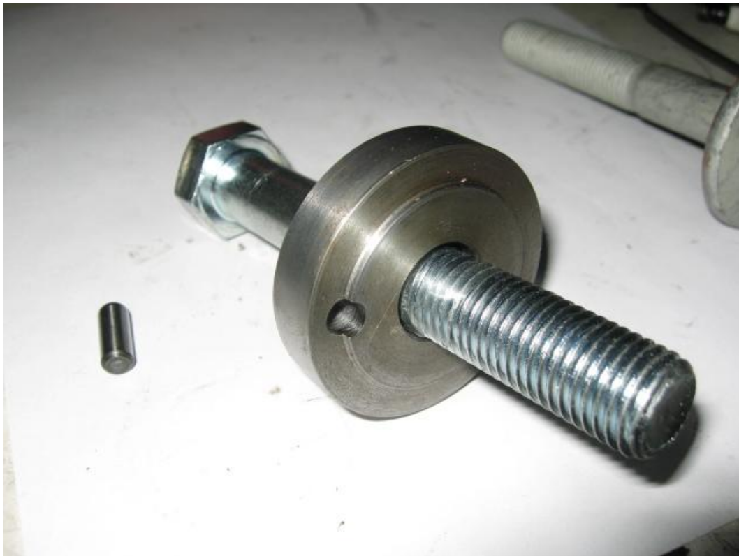
PIN FIXTURE WITH BOLT AND PIN
