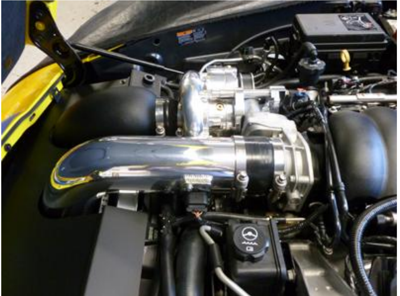
(INLET TRACT ASSEMBLED LS7 AND LS3)
