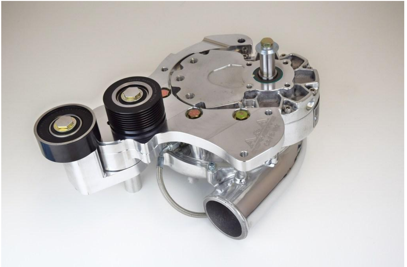
MAIN BRACKET BOLTED TO SUPERCHARGER LOCK THE TENSIONER IN THE OPEN (SLACK) POSITION
