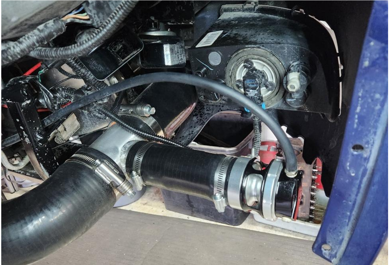
REAR VIEW OF BOV INSTALLED WITH HOSE C5-6-3 CONNECTED
