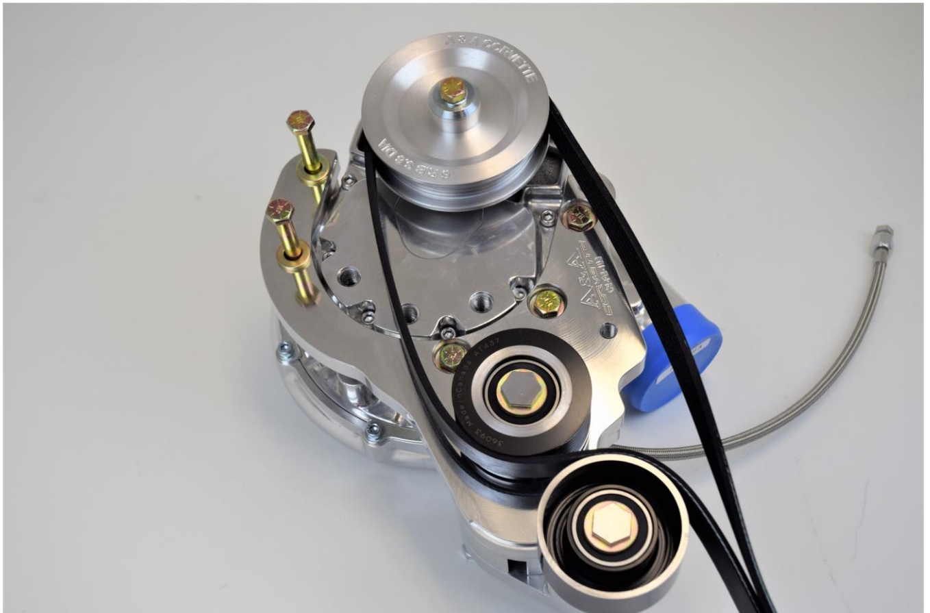
BELT SHOULD BE ROUTED LIKE THIS ON THE SUPERCHARGER BRACKET ASSEMBLY
