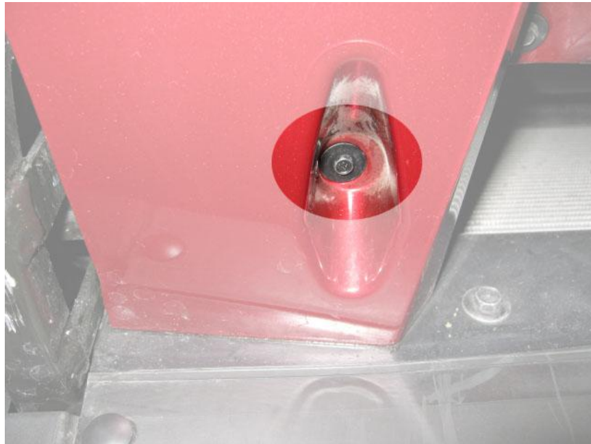
7mm SCREWS IN BOTTOM OF FASCIA
