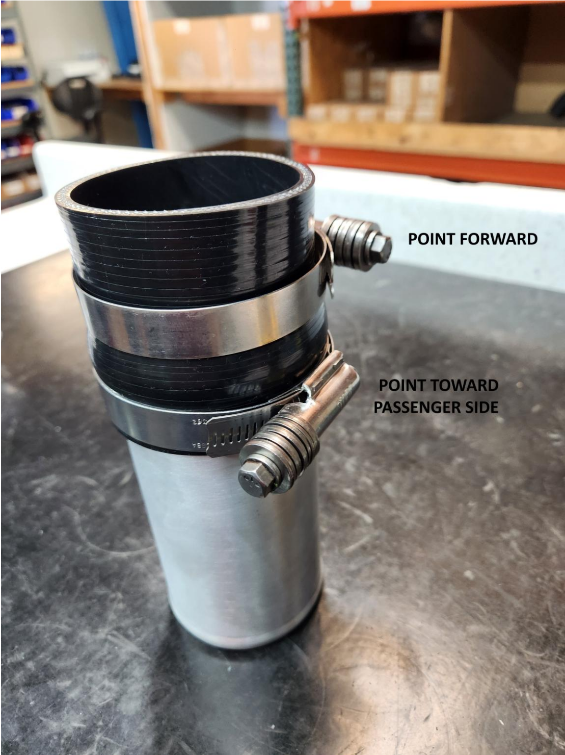
DISCHARGE TUBE CLAMP ORIENTATION
