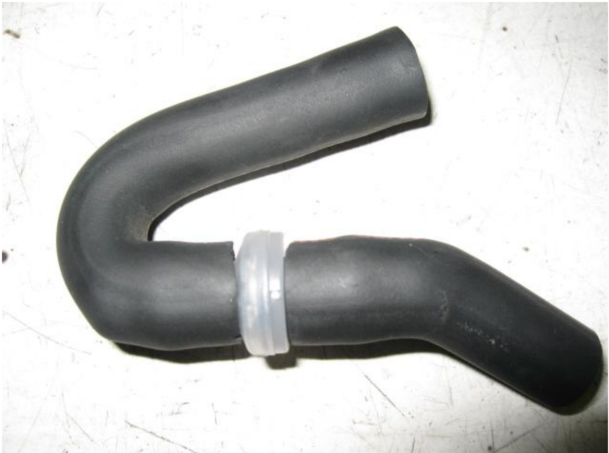
(CHECK VALVE INSTALLED IN PCV TUBE)
