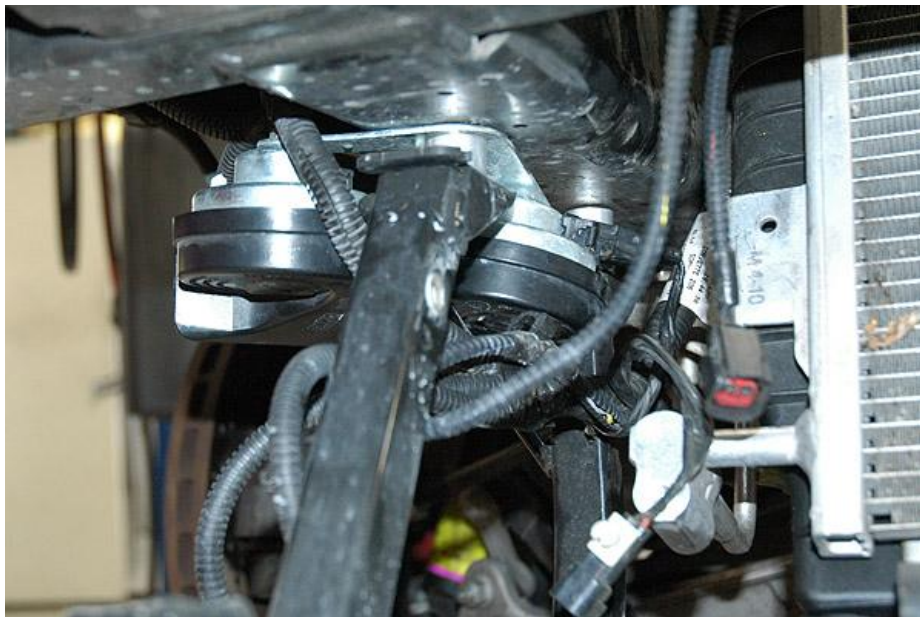
(HORN ASSEMBLY INSTALLED ON PASSENGER SIDE)
