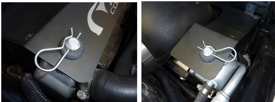
(LEFT AND RIGHT COTTER PINS INSTALLED)
