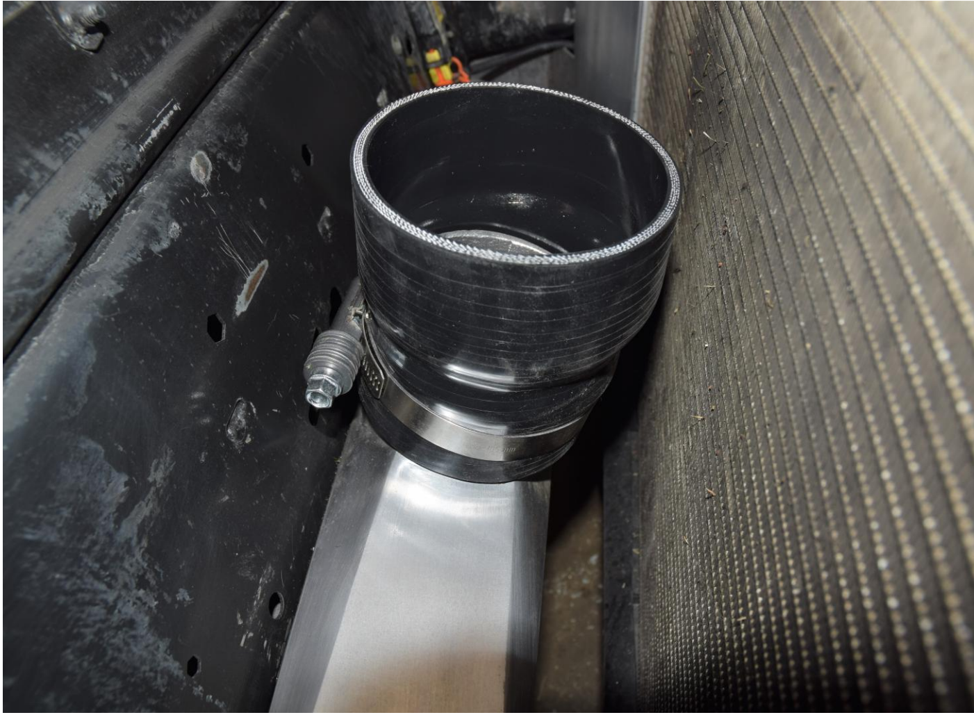
ANGLED COUPLER BETWEEN INTERCOOLER AND MAF TUBE
