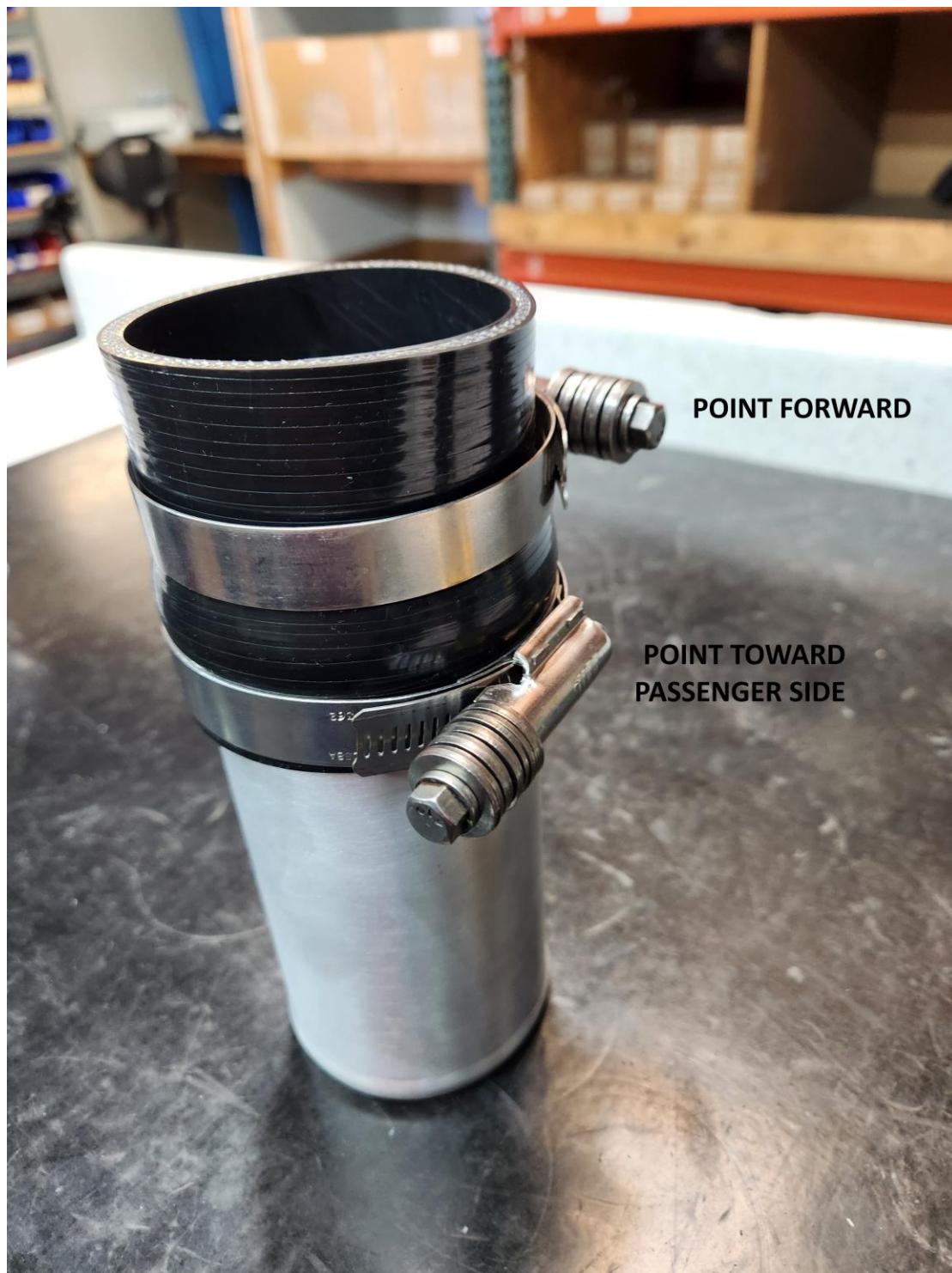
DISCHARGE TUBE CLAMP ORIENTATION
