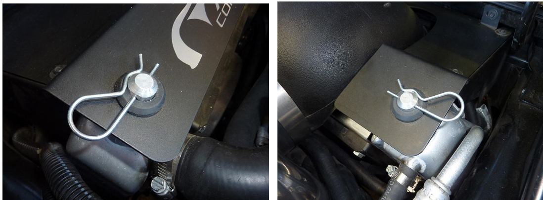
(LEFT AND RIGHT COTTER PINS INSTALLED)
