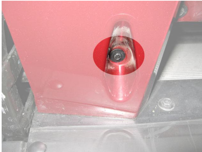
7mm SCREWS IN BOTTOM OF FASCIA
