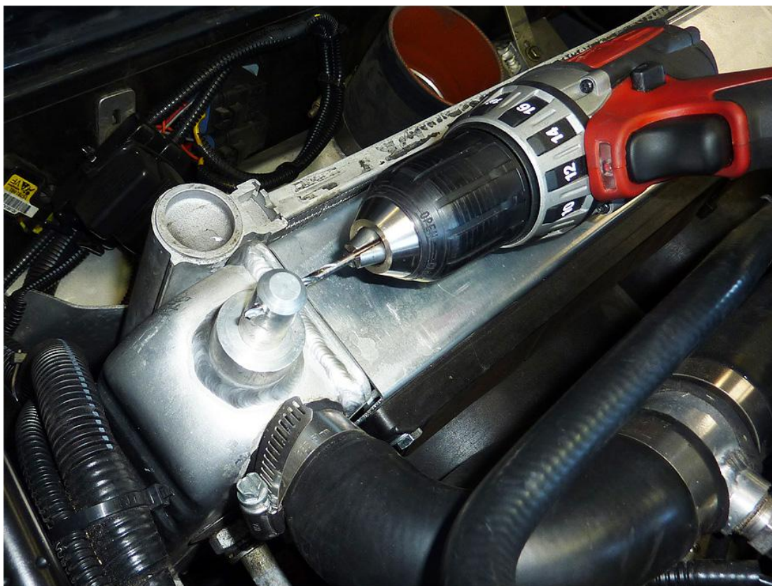
DRILL 1/8" HOLE THROUGH POST
