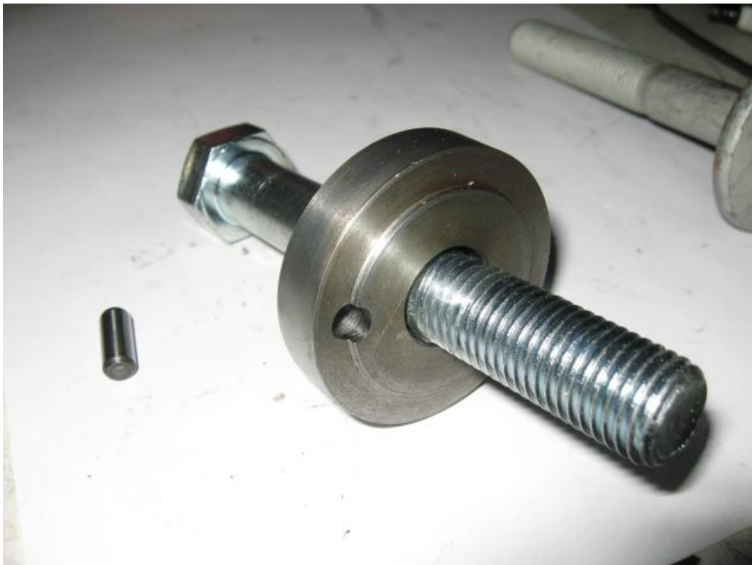
PIN FIXTURE WITH BOLT AND PIN
