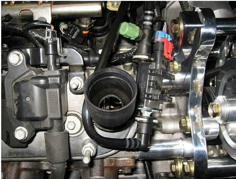
EVAP ASSEMBLY RELOCATED
