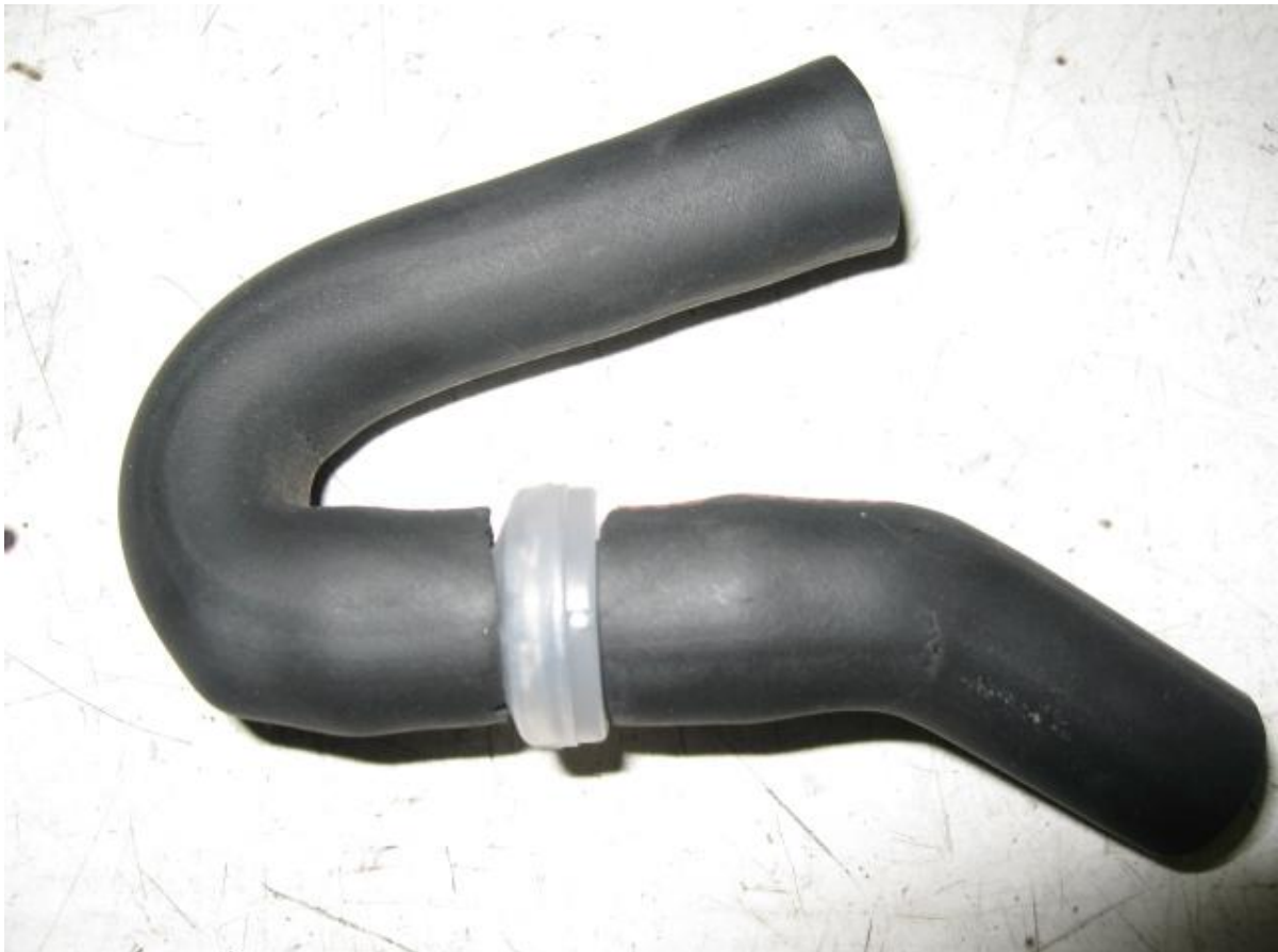
(CHECK VALVE INSTALLED IN PCV TUBE)
