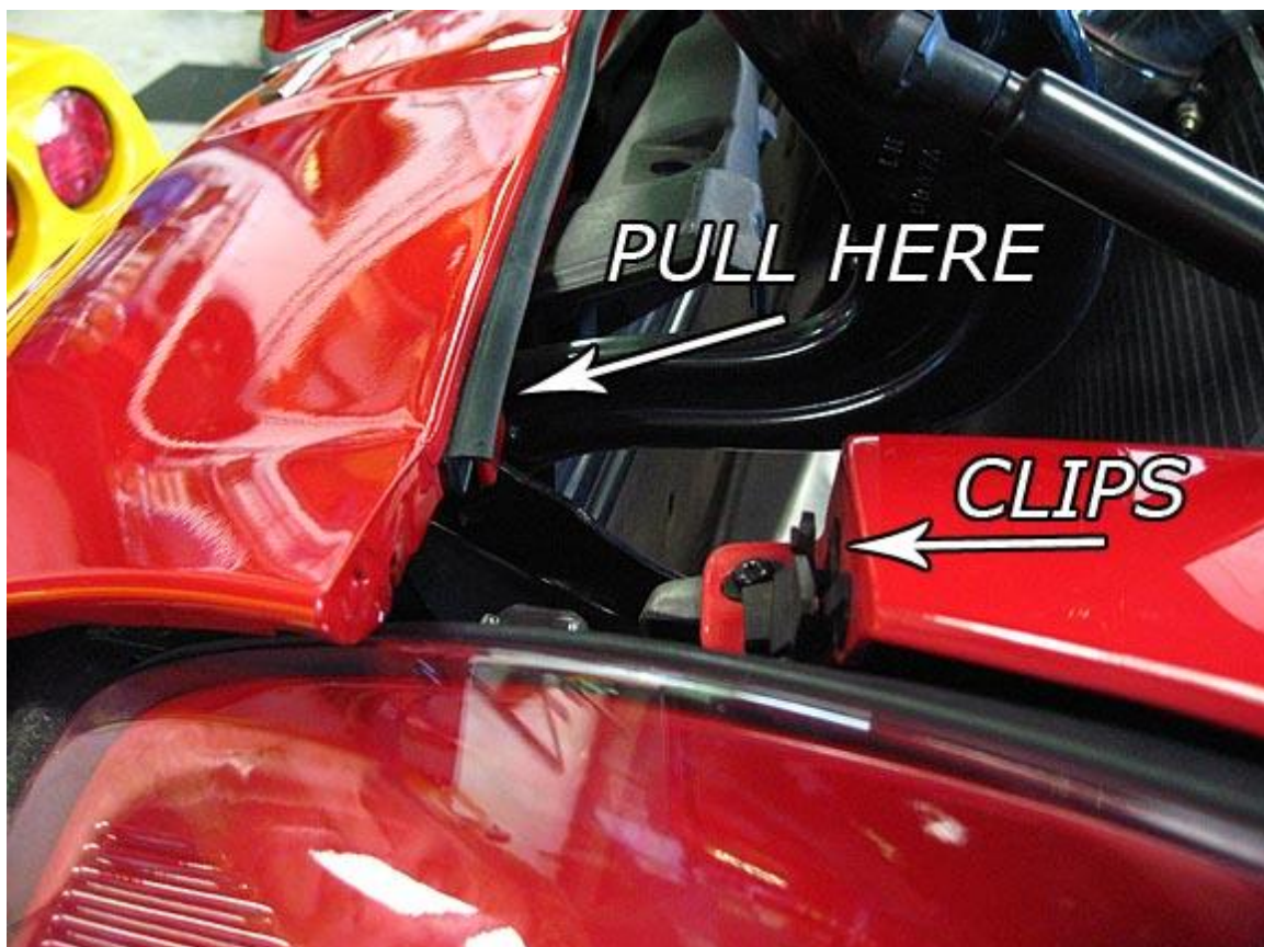
PULL STRAIGHT UP UNTIL THE FASCIA POPS OUT
