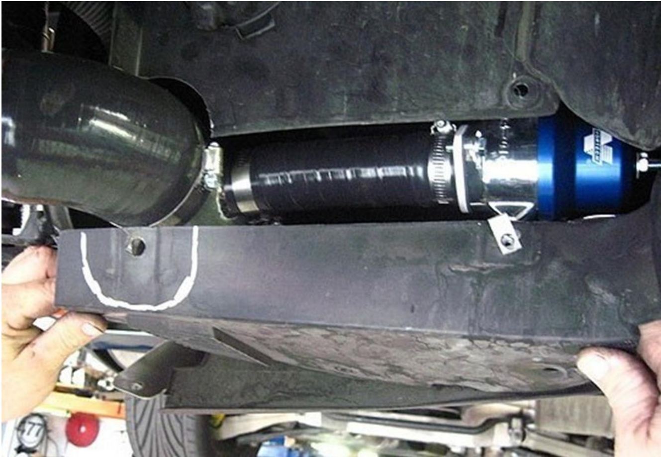
ENCLOSURE PANEL MARKED FOR TRIMMING
