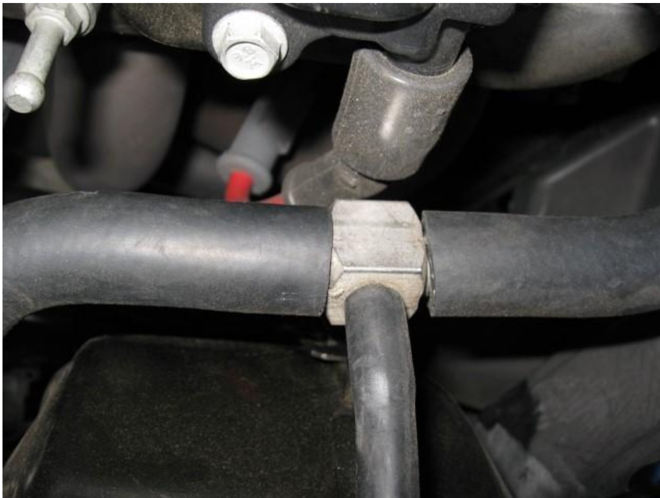
VACUUM T INSTALLED
