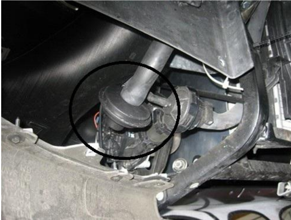
AIR FILTER INSTALLED IN PUMP INLET HOSE (FILTER STYLES MAY VARY)
