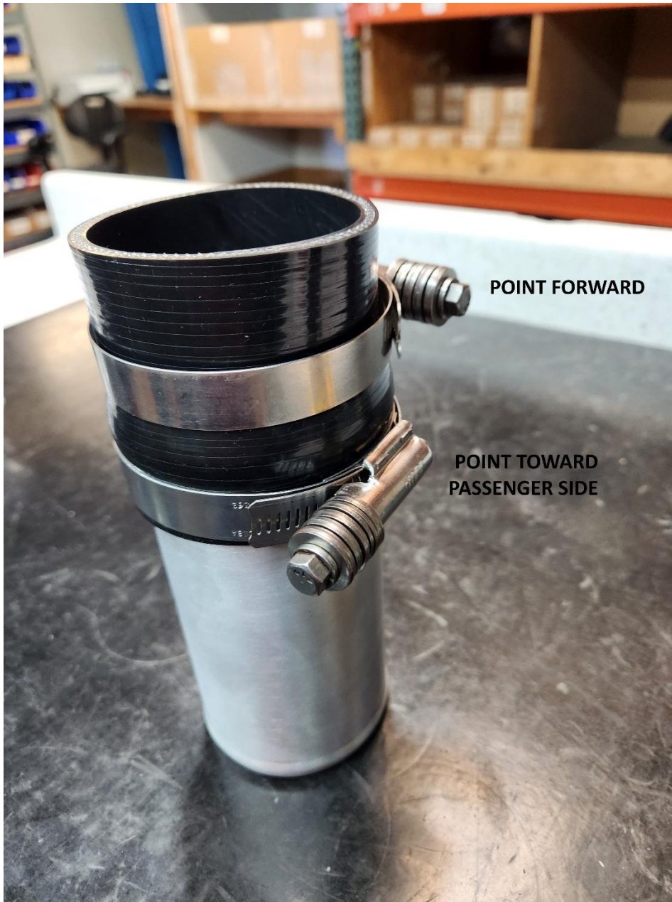
DISCHARGE TUBE CLAMP ORIENTATION
