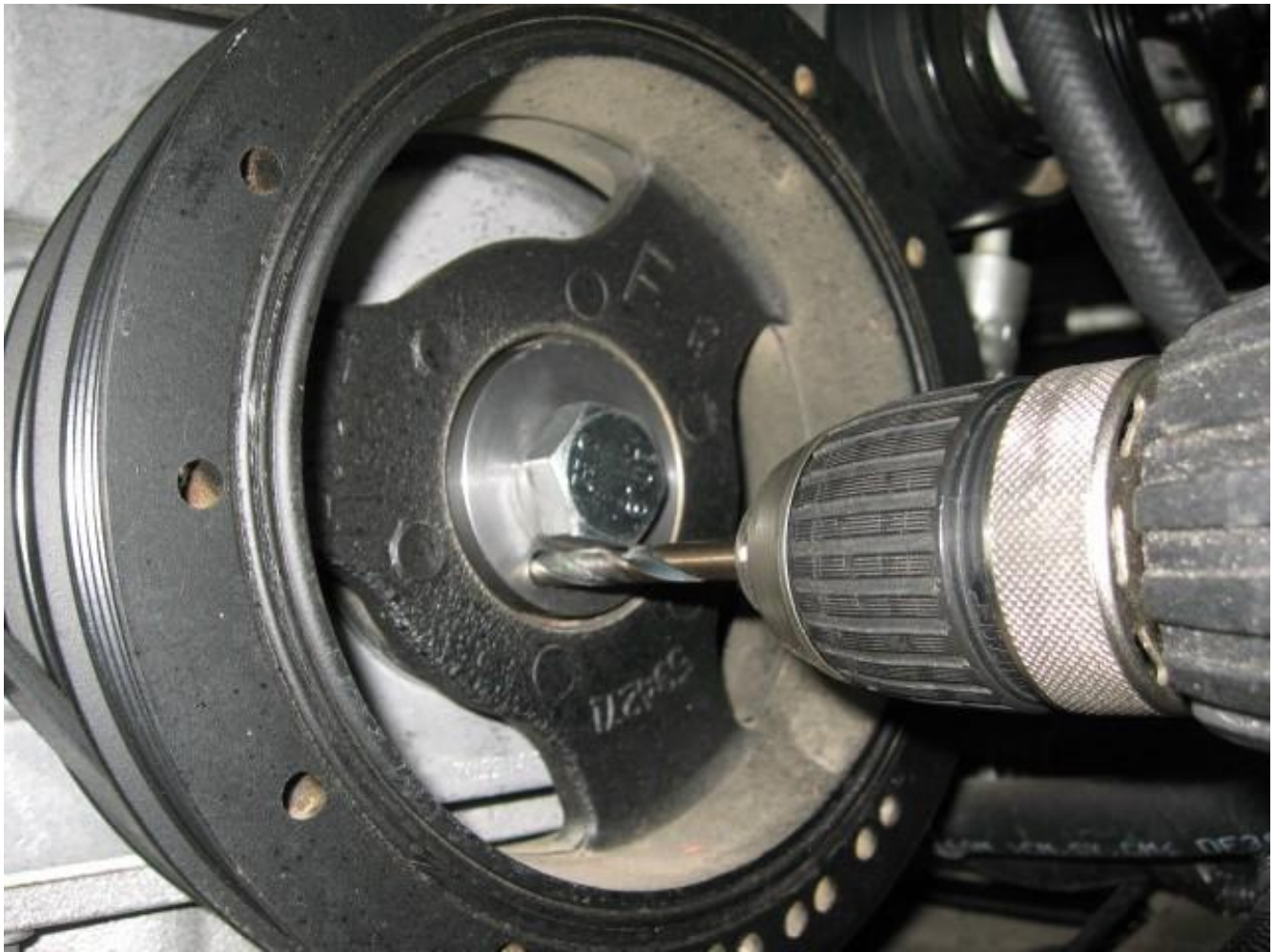
DRILLING CRANK AND BALANCER THROUGH PIN FIXTURE
