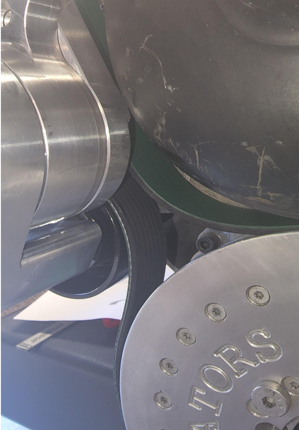
BELT COMING OFF TENSIONER AND UNDER BALANCER
