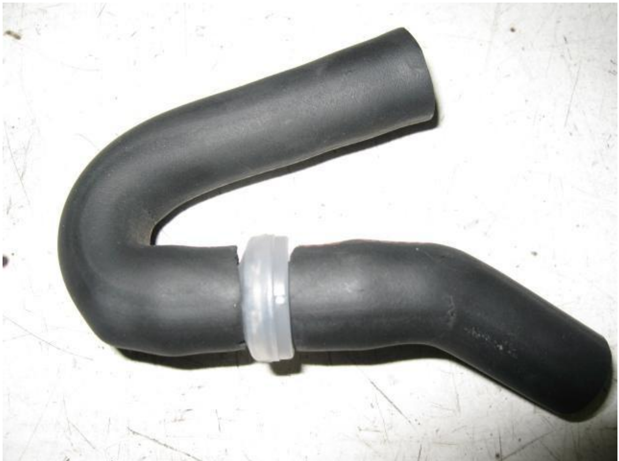
(CHECK VALVE INSTALLED IN PCV TUBE)
