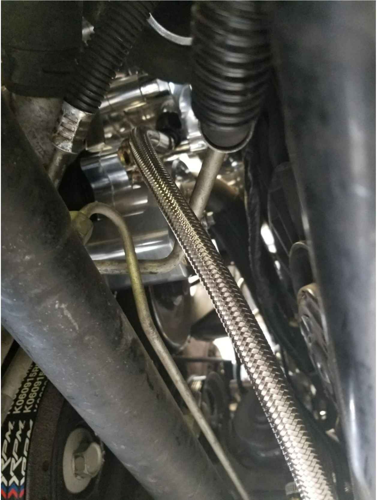
OIL-FED BLOWER DRAIN LINE ATTACHED
