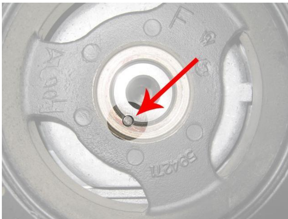
PIN INSTALLED IN CRANKSHAFT AND BALANCER
