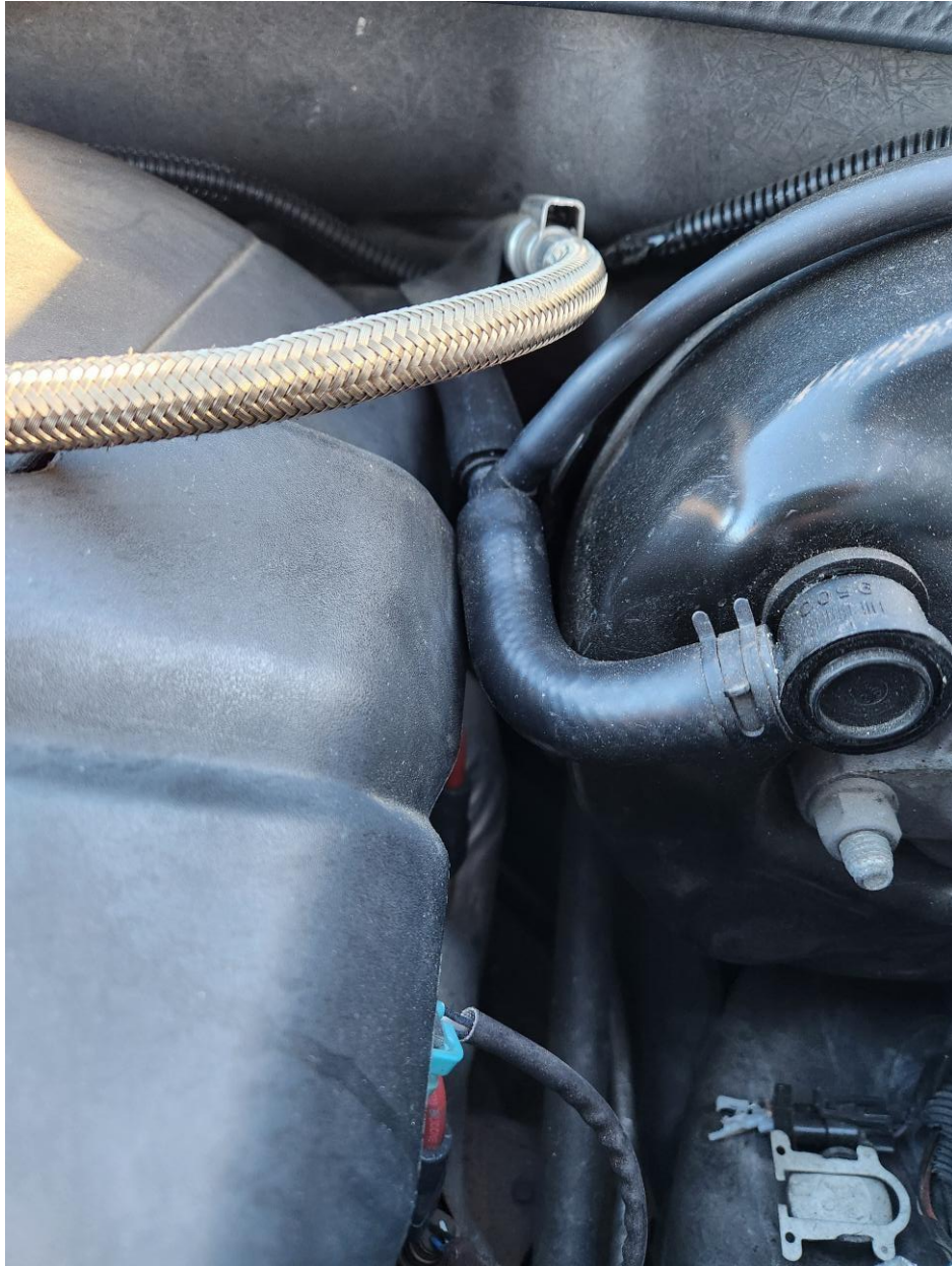
(VACUUM "T" INSTALLED IN BRAKE BOOSTER HOSE) (Note vacuum hose routed over the booster, away from the heat)
