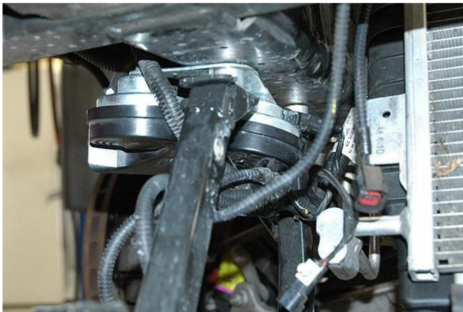
(HORN ASSEMBLY INSTALLED ON PASSENGER SIDE)
