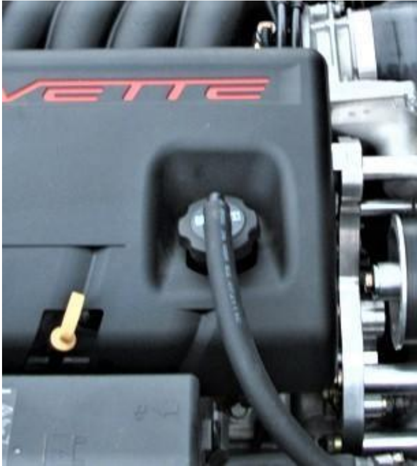
WET SUMP OIL CAP AND VENT LINE INSTALLED
