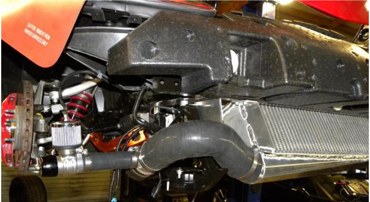
FRONT VIEW OF HOSE C6-2 AND BOV ASSEMBLY INSTALLED
